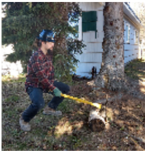
SWINGING + CHOPPING -Start with your hands spread apart on the tool handle -Bring the tool behind your back and over your shoulder -As the tool rotates over its center of gravity, your top hand slides down the handle -Let the tool do the work.
